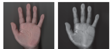
(left) A visible image of palm veins (right) An infrared image of palm veins
